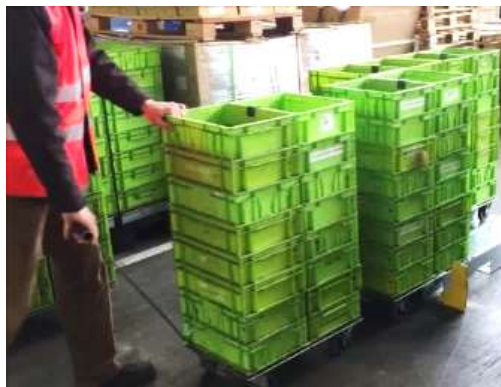
Rollis® trolleys are coupled with the towing hook ( L0005 )
