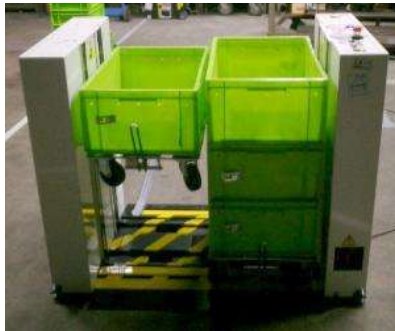
The Pile Lifter works with all container heights (maximum 320 mm high) Height is adjusted manually with a screw
