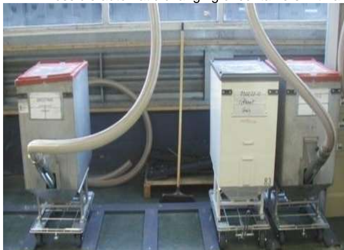
The small size Rollis enables to put several grades right on the injection molding machine
