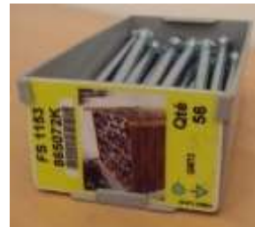
The Kanban card is housed in notches molded from the block ; Easy to grip and without hesitation thanks to its inclination
