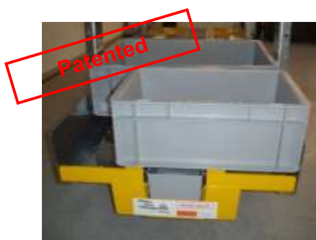
Empty container returned by guiding : no more stuck or dropped containers
