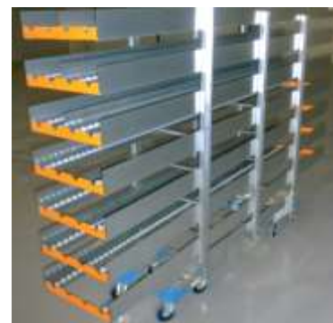
Rollis Skate ( LD0584 ) is used to move the racks, with 4 revolving wheels for lateral movements
