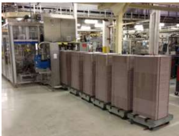
Rollis moving automatically into a forming machine
