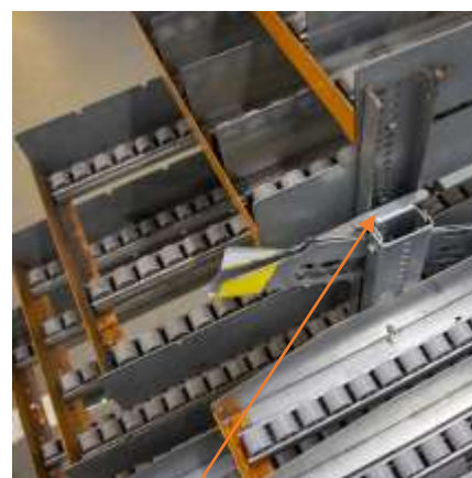
The spacer ( L0479 ) creates a space for the gutter between 2 Racks
