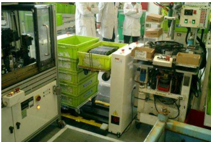
The return of empty container is outside of the line and does not make the operators path longer
