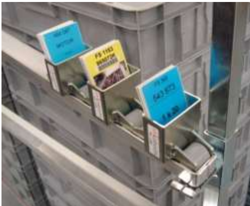
Cards arrive in the bucket in front of the operator in production order. The several cards show the references which have to be produced
