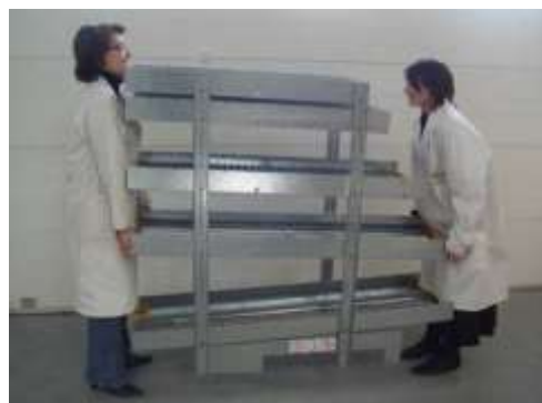
The self-carrying structure enables to move the Rack by hand in the consumption place on the assembling line
