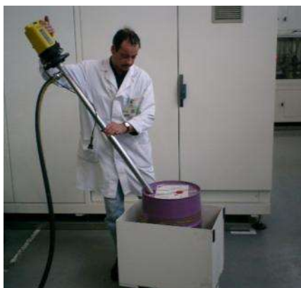
Introduction of the cannula, without risks of splattering
