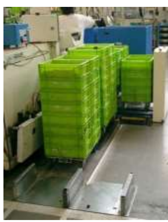
In / Out Kit to supply a Pile Lifter
