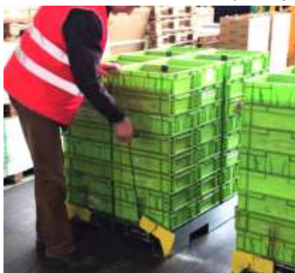
Locking latches are opened without bending down
