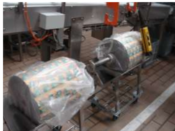
Support axle inserted at man height
