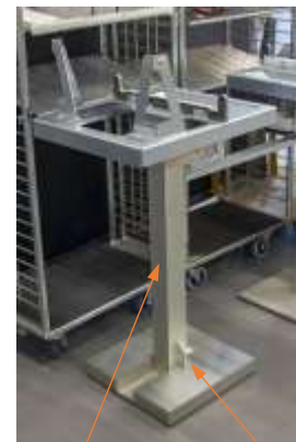
The layer (L0547) with ballast (L0288) hosts fitting template and tools
