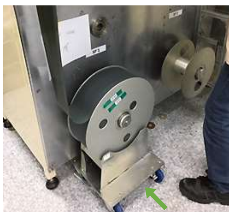
Lateral coil loading on a holder
