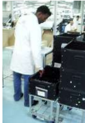
Boxes supply in square pitches ; the operator does not need to bend down
