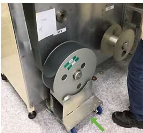
Lateral coil loading on a holder
