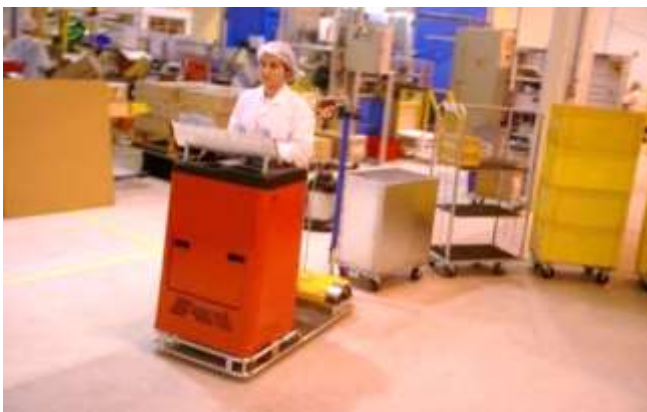
The Kanban desk is fixed in the top holes of the Ergomover. No adaptation is needed.
