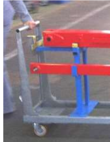
Ergonomic handle for manual manipulation
