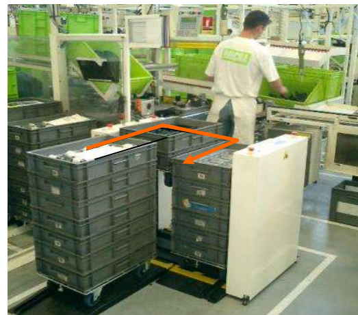
The pile lifter decreases the supply area and clears the work station
