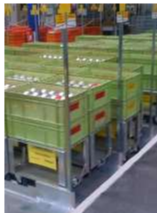
Ballasted heightened Rollis for copper circuit breaker poles L0111
