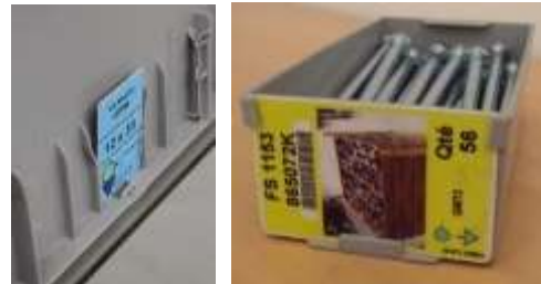
The Kanban card is housed in notches molded from the block ; Easy to grip and without hesitation thanks to its inclination
