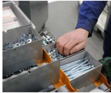
The mini-containers ergonomic width allows to grip the contents without any finger constraints
