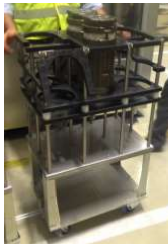
Rollis for quick change of injection tools
