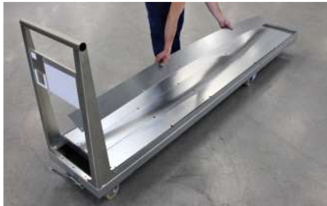
2 400 mm Transatlantic Rollis used as a shuttle for metal sheet transportation
