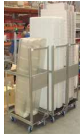
The rubberized carpet absorbs shocks while carrying fragile pieces
