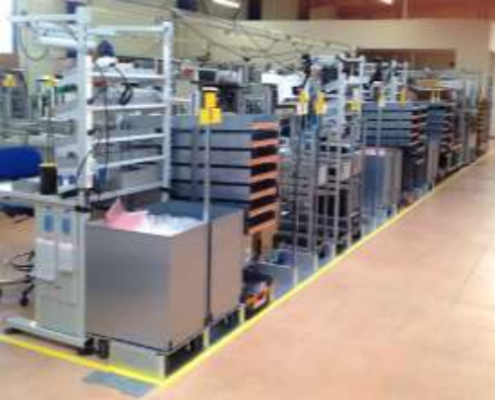
The line alternates between station and supply with containers in Rack and stacked on Rollis
