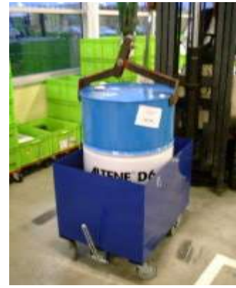
Loading with crowbar by hoist or forklift truck
