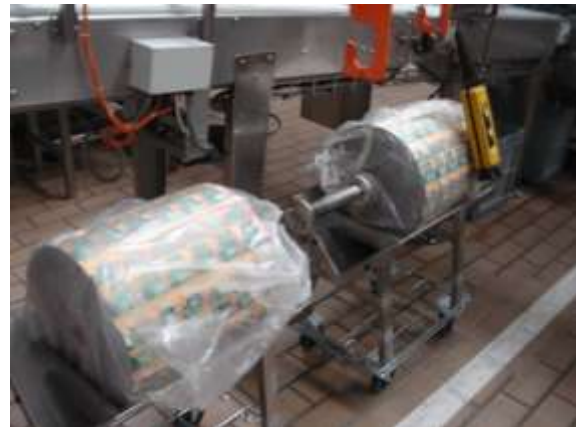
Support axle inserted at man height
