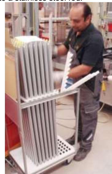
The operator « closes » the compartments as he fills the Benhur Rollis
