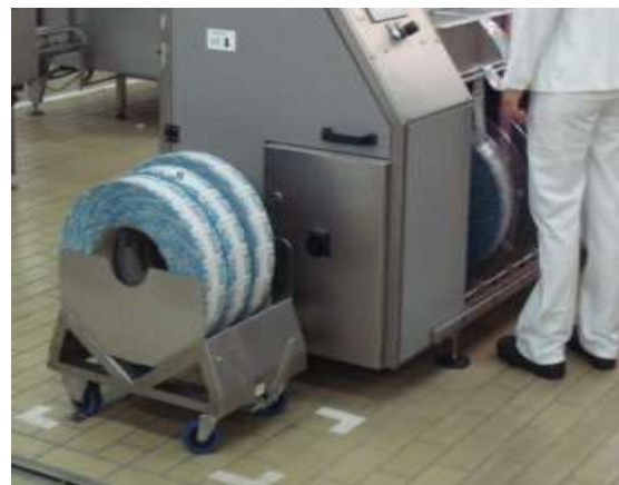
U Bobbin Rollis allows to receive several coils thanks to compartments
