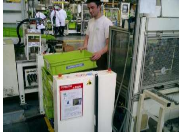
Switch of empty container onto the next pile
