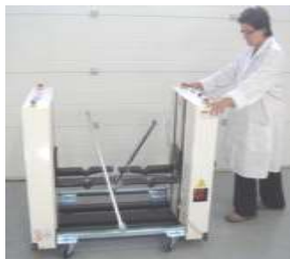
2 crutches (L0184) to move the Pile Lifter
