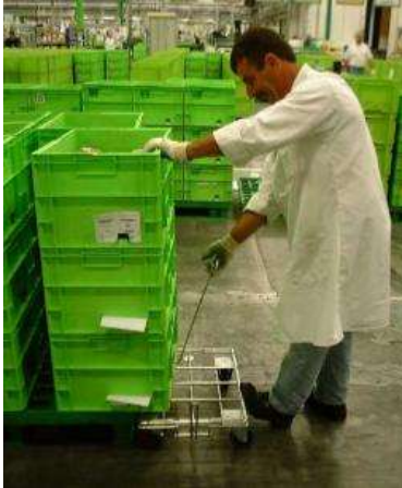
Manual transfert from pallet to Rollis®
