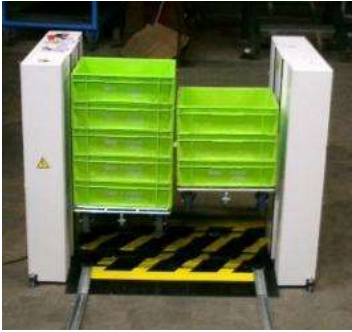
The Pile Lifter works with all container heights (maximum 320 mm high) Height is adjusted manually with a screw
