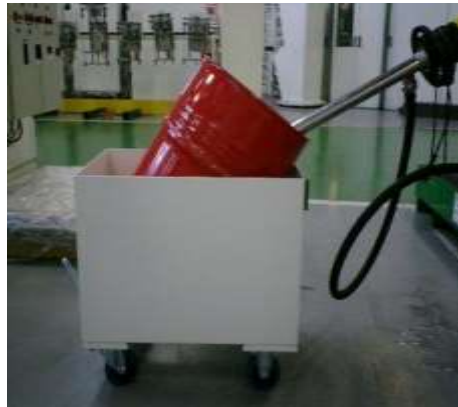
The system allows to tilt the barrel for complete emptying
