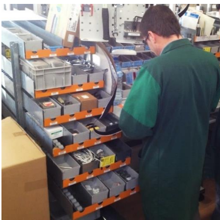
Ergonomic pieces handling thanks to the offset of the layers in organ keyboard
