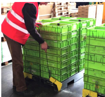
Locking latches are opened without bending down
