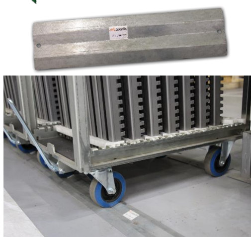
The Rollis floor positionner blocks the 2 front wheels
