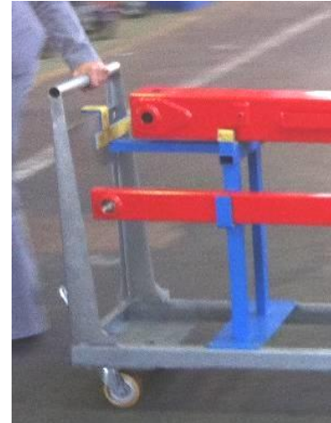
Ergonomic handle for manual manipulation
