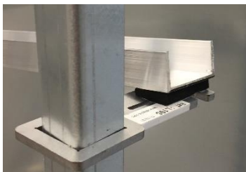
Rail fixed on holding brackets ( L0195 ) with double-sided sticky foam
