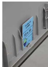
The Kanban card is housed in notches molded from the block ; Easy to grip and without hesitation thanks to its inclination
