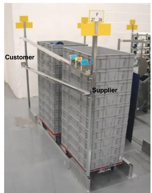
Launching Rail ( L0196 ) fixed by 2 holding brackets ( L0195 ) on storage units poles
