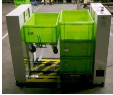
The Pile Lifter works with all container heights (maximum 320 mm high) Height is adjusted manually with a screw
