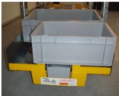
Empty container returned by guiding: no more stuck or dropped containers
