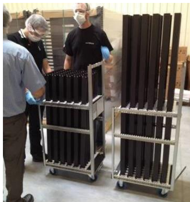
Dividers protect the paint of pieces against shocks
