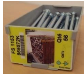
The Kanban card is housed in notches molded from the block; Easy to grip and without hesitation thanks to its inclination
