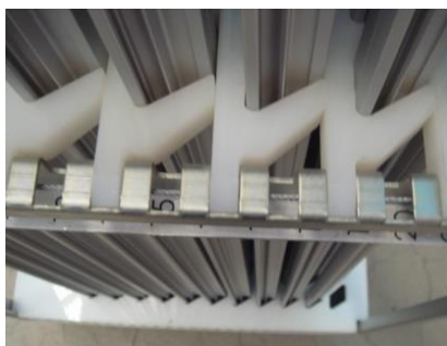
Stainless steel rod ( L0069 ) inserted in the rack and through the dividers
