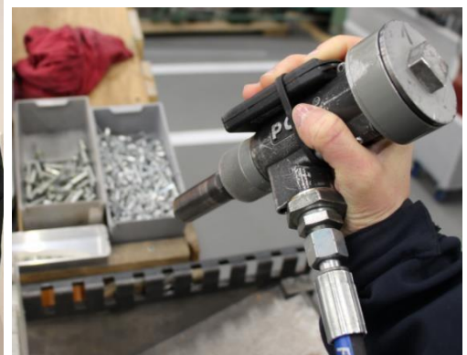
Amended riveting tool: Lightweight (without accumulation of rivet tails) Ergonomic (right wrist taking)
