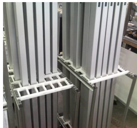
The divider holds the pieces ; it is inserted in anumbered rack
