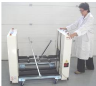
2 crutches (L0184) to move the Pile Lifter
