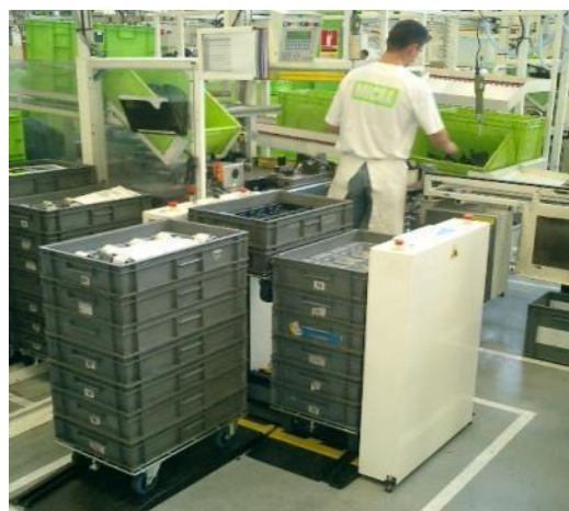
The pile lifter decreases the supply area and clears the work station
