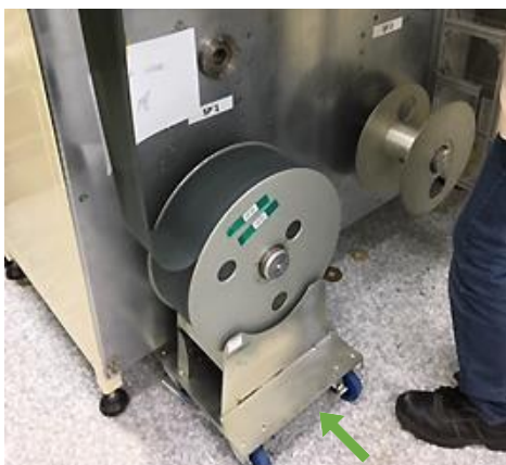
Lateral coil loading on a holder
