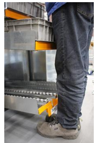
Ergonomic design: the operator can be as close as possible to the pieces
