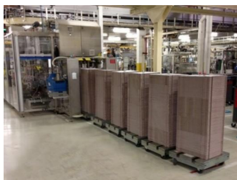
Rollis moving automatically into a forming machine
