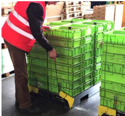
Locking latches are opened without bending down
