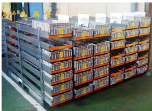
Less than 1 350 mm high is ergonomic height which enables to see the whole workshop
