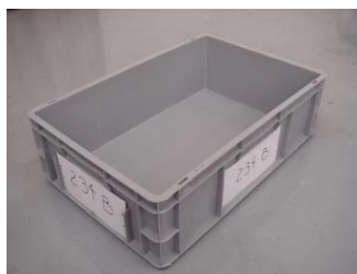
400 x 300 container: Storage identification on any side
