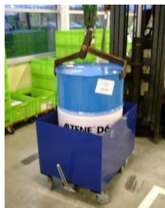
Loading with crowbar by hoist or forklift truck
