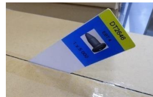
Card can be inserted directly into the cardboard slots to identify its contents. Information on Kanban is always visible
